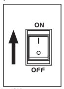
3. Turn the fuel tap into position 'ON'.
