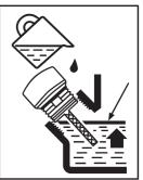
Please fill in the engine oil (approx. 0.55 l) until the oil level reaches the upper edge of the filler neck.
